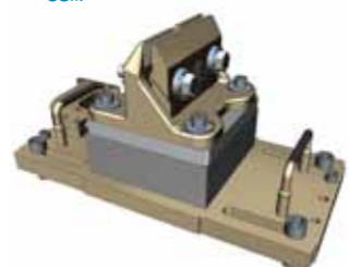
MIMS clamp assembly with multi axis piezo-electric load cell.
